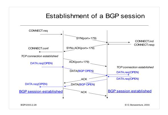
Usually, a BGP session can only be established between two manually configured peers. Each peer needs to be configured with the IP address and the AS number of the remote peer.
