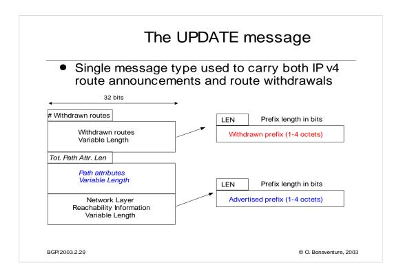
This format is used when BGP carries IP v4 routing information. With the MultiProtocol extensions, BGP can be used to carry different types of addresses instead the same BGP session (e.g. IP v6, RFC2547 VPNs, MPLS labels, or IP Multicast routing information). See e.g. :
