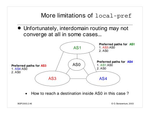
In practice, the exchange of BGP UPDATE messages will cease due to the utilization of timers by BGP routers and the routing will stabilize on one of the two stable route assignments.
