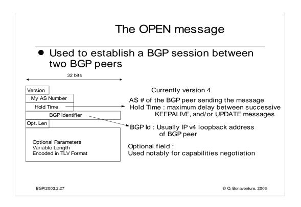
Inside the OPEN message, and also in the Path attributes of the UPDATE message, the AS number is encoded as a 16 bits field. This limits the number of Ases in the global Internet. Given the rapid growth in the number of AS present on the Internet, the AS space could become completely full within a few years.
