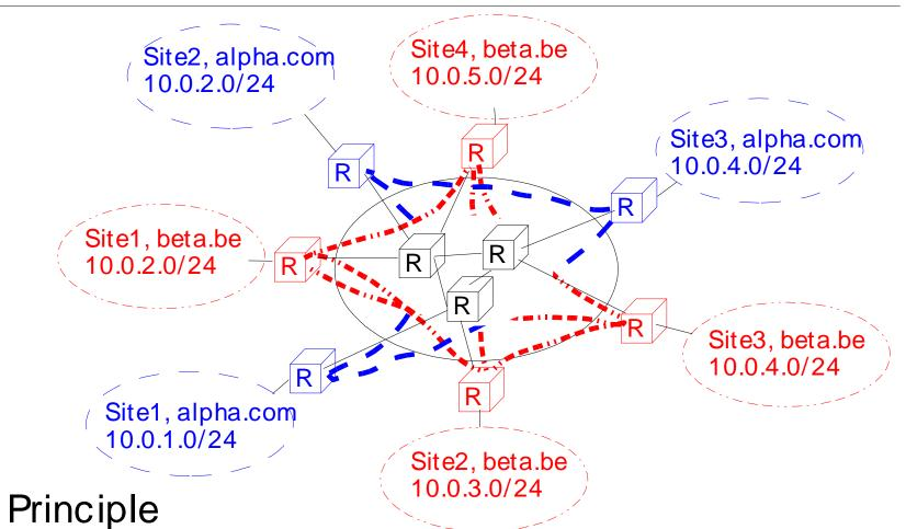
Manually create LSPs between customer routers from VPN sites through MPLS backbone
