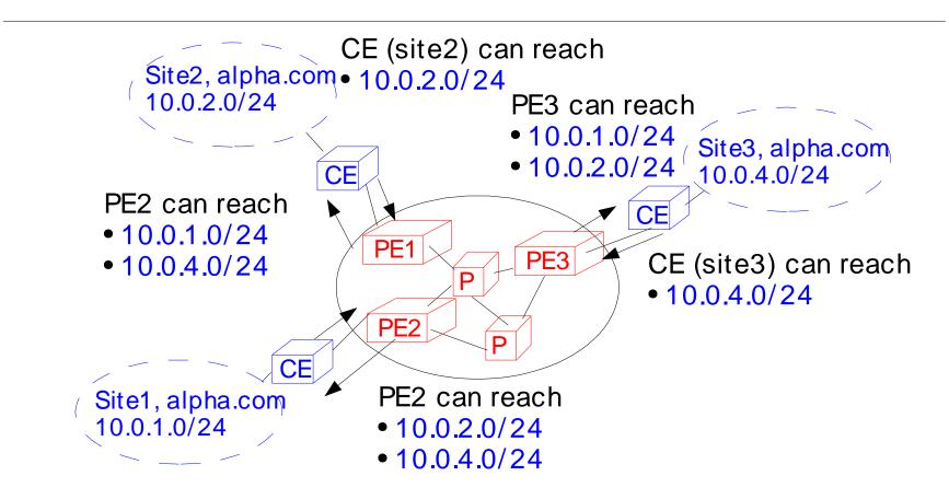
In the backbone, all P and PE routers know ISP backbone topology by using the normal IGP
