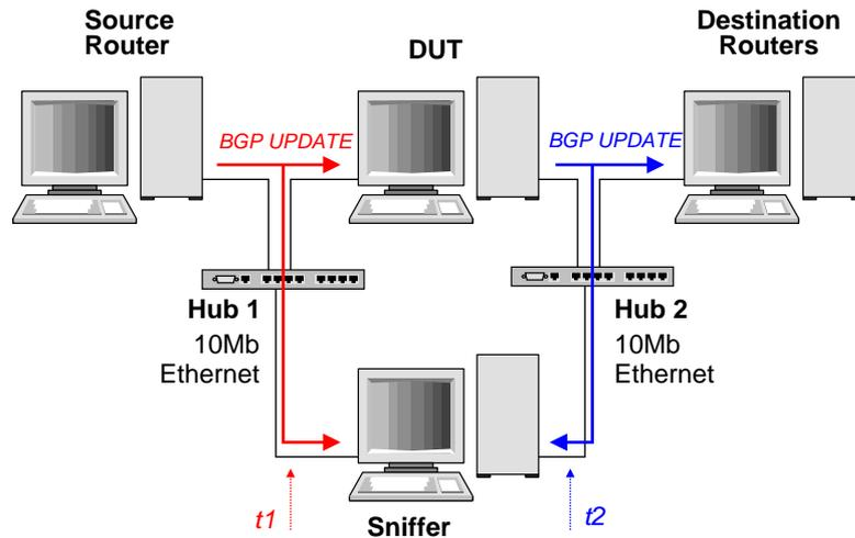
Fig. 6. Measurement testbed.
